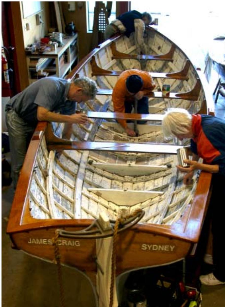
ribs were repaired, the bottom stripped and repainted, and the inside cleaned and sanded. I only became involved with the final sanding and painting inside, with the help of many willing Sunday volunteers.
